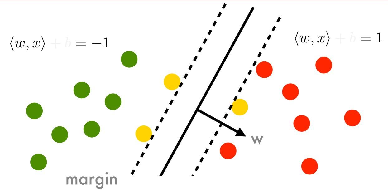
$$\frac{\langle x_{+} - x_{-}, w \rangle}{2 \|w\|} = \frac{1}{2 \|w\|} \left[ \left[ \langle x_{+}, w \rangle + b \right] - \left[ \langle x_{-}, w \rangle + b \right] \right] = \frac{1}{\|w\|}$$
