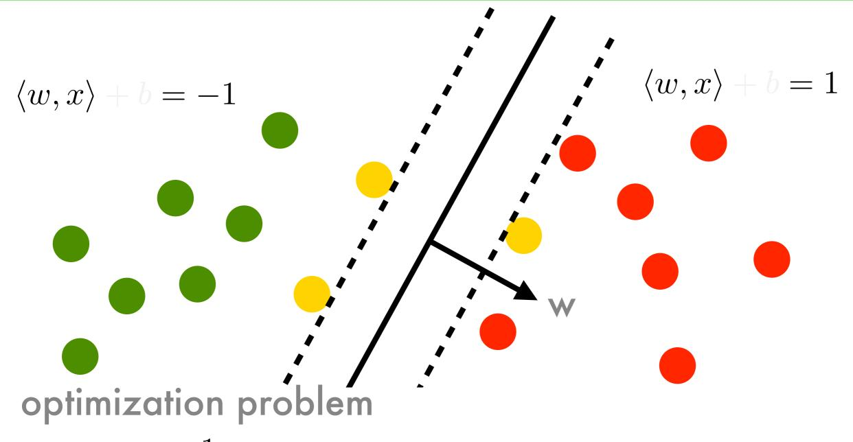
$\underset{w,b}{\operatorname{minimize}} \frac{1}{2} \left\| w \right\|^2 \ \text{subject to} \ y_i \left[ \langle x_i, w \rangle + b \right] \geq 1$
