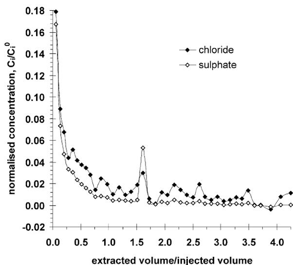
Fig. 2. Chloride and sulphate breakthrough curve from the extraction phase of the push-pull test. Normalised tracer concentrations have been corrected for background concentrations. The large peak for which the normalised sulphate concentration surpasses the normalised chloride concentration corresponds to the period when pumping was momentarily interrupted.
