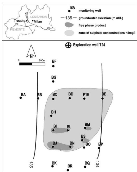
Fig. 1. Map of the crude oil contaminated site near Trecate, Novara, Italy. The site location is in the inset. Note the location of the oil well T24, source of the contamination. The push-pull test was conducted in well BC.
