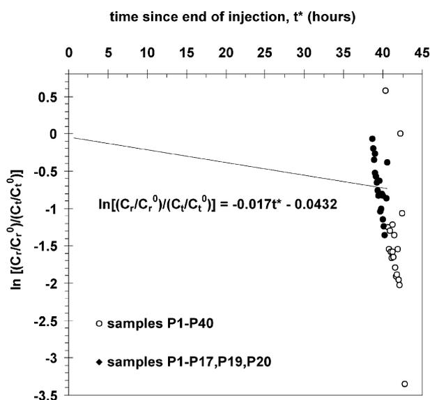
Fig. 3. Example of fit of first-order degradation model (solid line) [Eq. (3)] to field data. Selected data points (samples P1–P19 and P20) that correspond to when tracer concentrations were above background levels and when conditions were anaerobic, were used to fit the model.
