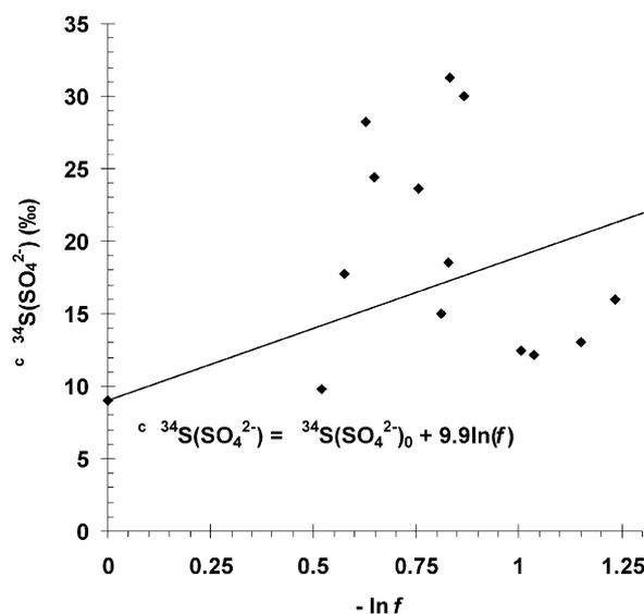
Fig. 5. Rayleigh distillation model (solid line) fit using least squares linear regression to corrected  $\delta^{34}\text{S}(\text{SO}_4^{2-})$  values. The isotopic enrichment factor  $\epsilon$  is given by the slope of the line.  $f$  is the fraction of unconsumed reactive sulphate tracer remaining. Data from early samples (P1–P4) for which  $\text{S}^{34}$  enlightenment was measured have been neglected in the model.
