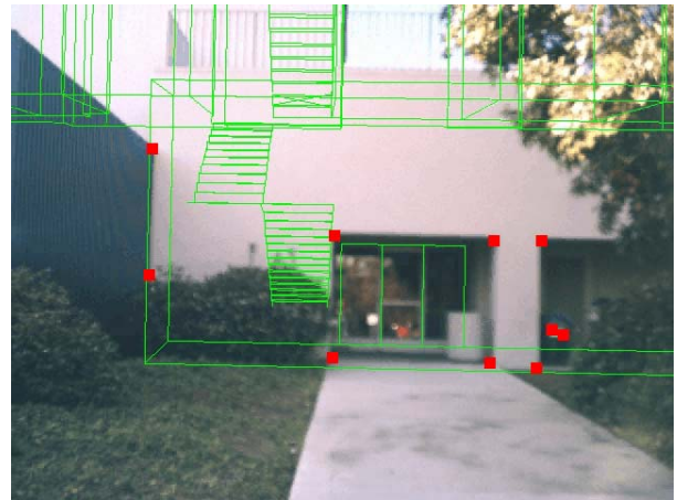
Figure 1: This image shows the feature points that have been dynamically picked for this building. Once the feature points have been found, the structure and its orientation can be found. As a result, useful information such as building schematics can be overlaid on top on the building itself.
