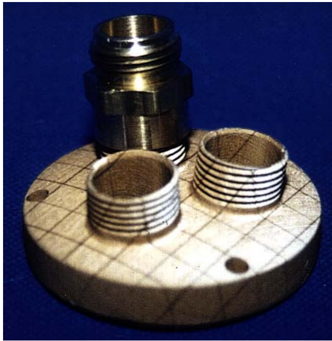
Figure 5: Finished Part with a Fitting on One of the Threads
