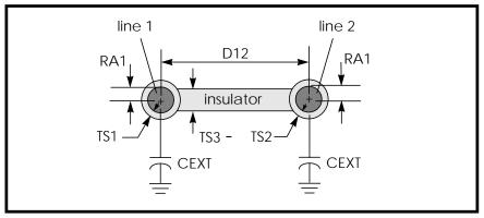
Figure 21-17: Geometric Twinlead, DLEV=1, with Insulating Spacer
