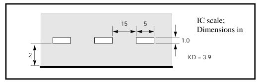
Figure 21-28: shows the IC-scale coupled line geometry.
