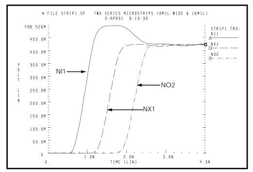
Figure 21-43: Waveforms in Mismatched Transmission Line Structure
