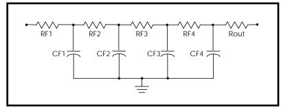
Figure 21-40: Circuit Diagram of an RC Filter
