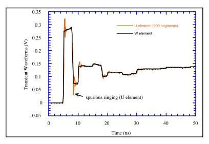
Figure 21-45: Fig. 1. Spurious ringing in U element, four-conductor lossy line
