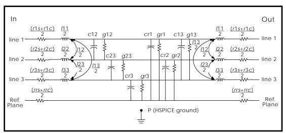
Figure 21-19: Precomputed Components for Three Conductors and a Reference Plane
