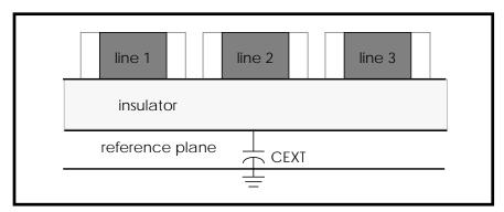
Figure 21-12: Planar Transmission Line, DLEV=1, Microstrip
