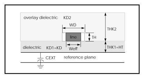
Figure 21-14: Planar Transmission Line, DLEV=3, Overlay Dielectric
