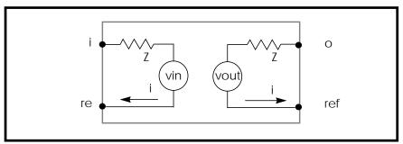
Figure 21-5: Ideal Element Circuit
