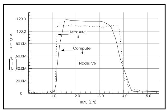
Figure 21-25: Measured Versus Computed Backward Crosstalk Response
