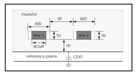
Figure 21-11: Planar Transmission Line, DLEV=0, Sea of Dielectric
