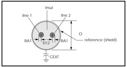
Figure 21-18: Geometric Twinlead, DLEV=2, Shielded
