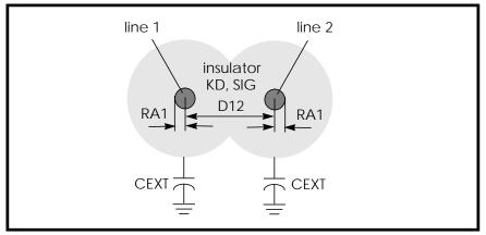
Figure 21-16: Geometric Embedded Twinlead, DLEV=0, Sea of Dielectric
