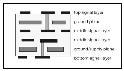
Figure 21-38: Six-Layer Printed Circuit Board
