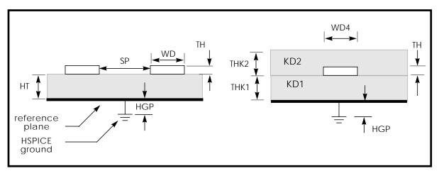
Figure 21-9: U Element Conductor Dimensions
