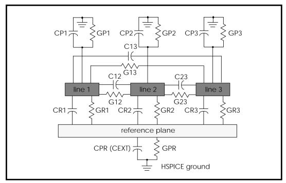
Figure 21-21: Single-Lump Circuit Capacitance
