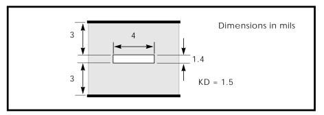
Figure 21-36: Stripline Geometry Used in MCM Technology
