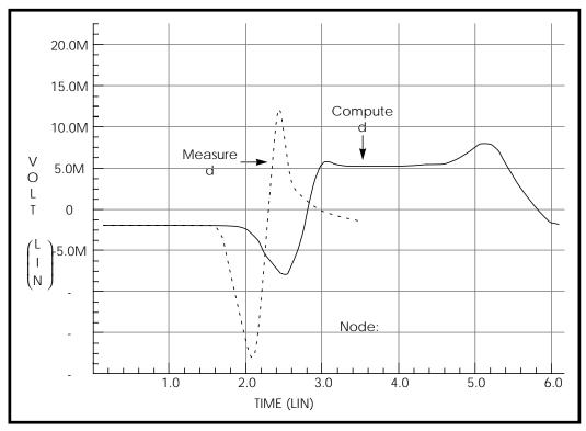
Figure 21-26: Measured Versus Computed Forward Crosstalk Response
