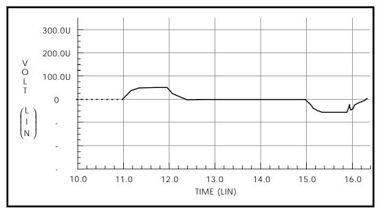
Figure 21-33: Computed Furthest Coupled-Line Response
