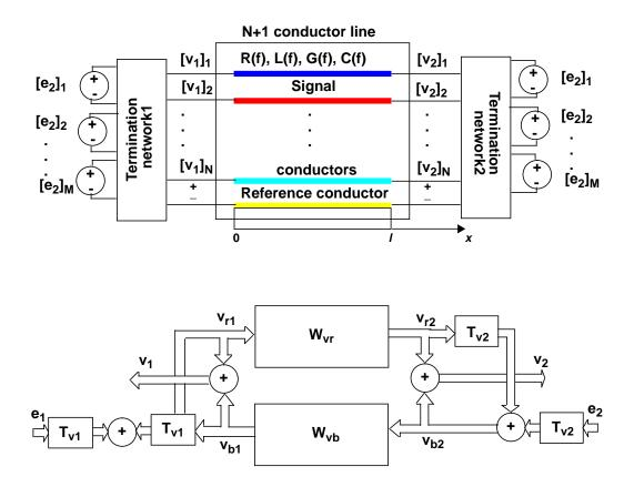
Figure 21-49: System model for transmission lines.
