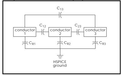
Figure 21-35: Conductor Capacitances for Example 2
