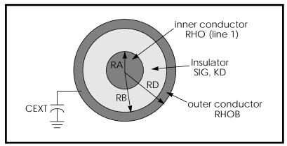
Figure 21-15: Geometric Coaxial Cable
