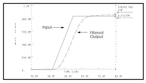
Figure 21-41: Multistage RC Filter Input and Output
