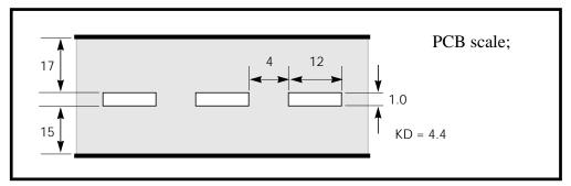
Figure 21-22: Three Coupled Striplines (PCB Scale)
