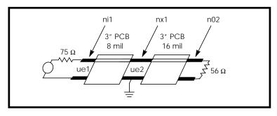
Figure 21-42: Mathematical Transmission Line Structure
