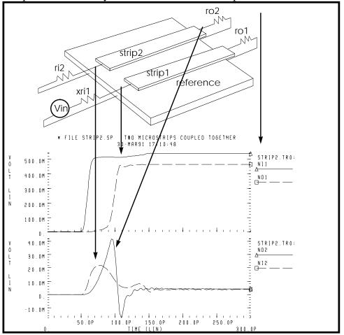
Figure 21-39: Two Coupled Microstrips Geometrically Defined as LSI Metallization
