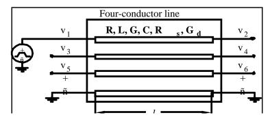
Fig. 3. Four-conductor line.
