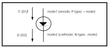
Figure 4-3: Diode (node1, node2)
