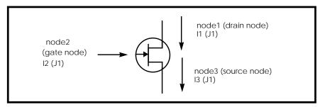
Figure 4-4: JFET (node1, node2, node3) - n-channel
