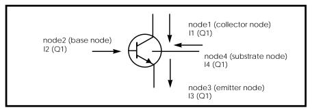
Figure 4-5: BJT (node1, node2, node3, node4) - npn
