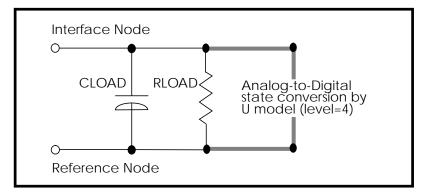
Figure 5-8: Analog-to-Digital Converter Element
