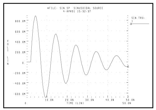
Figure 5-2: Sinusoidal Source Function
