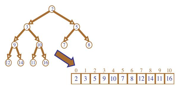
To insert a new value into a heap the value is first added to the end. This preserves the complete binary tree property, but not the heap ordering. To fix the ordering, the new value is *percolated* into position. It is compared to its parent node. If smaller, the node and the parent are exchanged. This continues until the root is reached, or the new value
