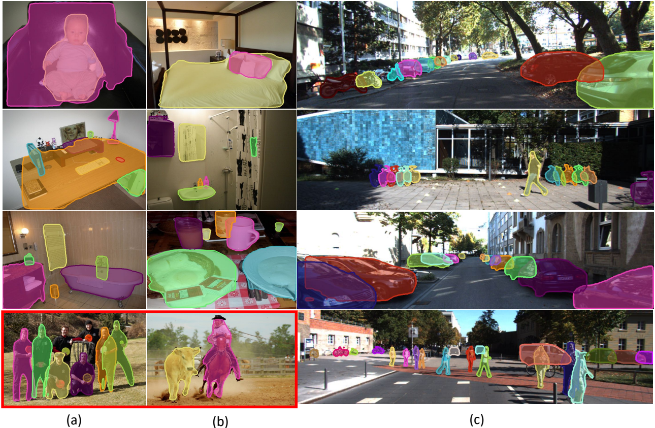
Figure 7. Qualitative results for amodal instance segmentation on COCOA-test are shown in (a) and (b), and on KINS-test in (c). All of them are successful cases except the failure cases are marked red. The first failure case is about incomplete person detections and the second failure case is about merging masks of a person and horse.
