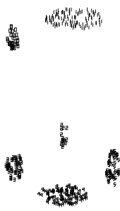
Figure 4: Clusters as found by a mixture of Gaussians with a uniform background component for clutter removal
