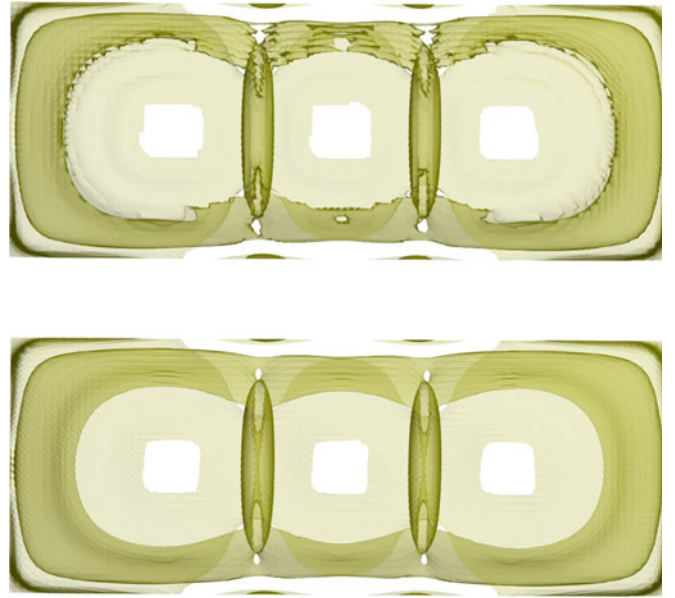
Fig. 3. This figure compares the neutral surface of the three ball simulation using the Marching Tetrahedra method (top) and the A-patches method (bottom). Notice that not only does the A-patches method better preserve geometry details such as the outline of the holes, it also reduces the topological errors caused by the Marching Tetrahedra method.
