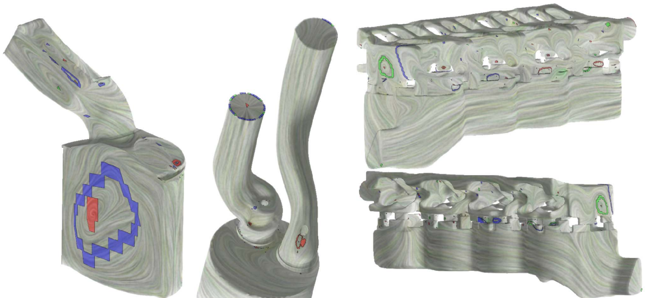
Fig. 17. This figure provides the Morse decompositions of the gas and diesel engine simulations, and cooling jacket simulation using the refinement framework without setting \tau_{max} . The analysis takes about 213, 1,012, and 4,524 s for these data sets, and returns MCGs with 63, 210, and 265 Morse sets, respectively.
