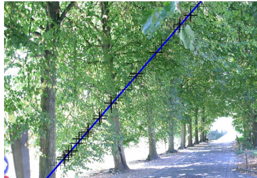
Figure 5: Example of how matching ambiguity can still exist even with 1-D epipolar constraints.
