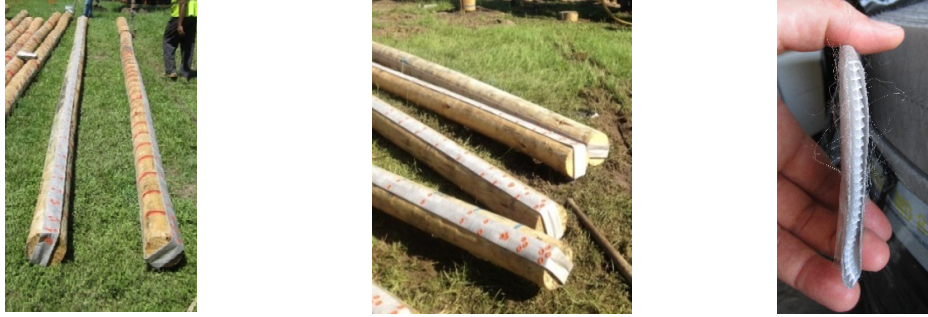
Figure 2. Drained timber piles and PVDs used in this study
