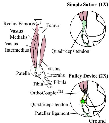
Fig. 1: Cross section of the knee joint. The top close-up shows the normal knee without an implant. The bottom close-up shows the knee with a pulley implanted for force scaling.
