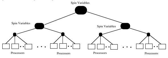
They are divided into groups and each group spins on a separate variable. The last processor in each group to arrive at the barrier must "report" to a higher level in the tree and spin on a new variabl. When we reach the root of the tree which indicates the completion of the barrier, the children of the root are released. These children in turn release their children, propagating the release down the tree.
