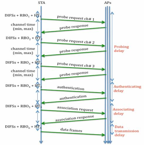
Fig. 1. Total delay between probe request frame and data frame.
