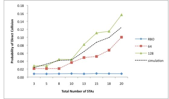
Fig. 8. Probability of direct collision vs. number of STAs and backoff slots.
