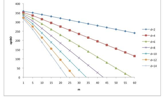
Fig. 3. Optimum backoff slots as function of  $m$  and  $d$ .
