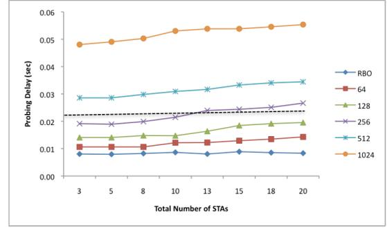
Fig. 7. Probing delay vs. number of STAs and backoff slots
