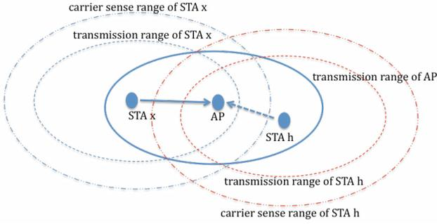
Fig. 4. Hidden node collision in the three-entity topology.
