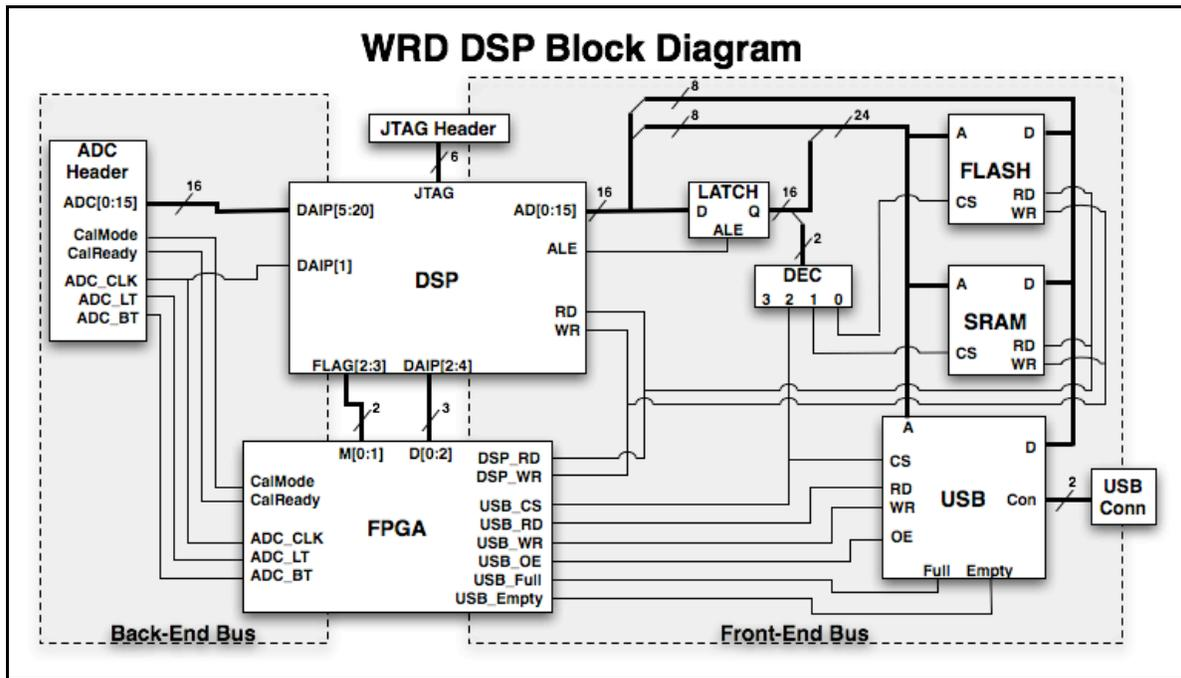
Figure 2. A block diagram of the DSP component.
