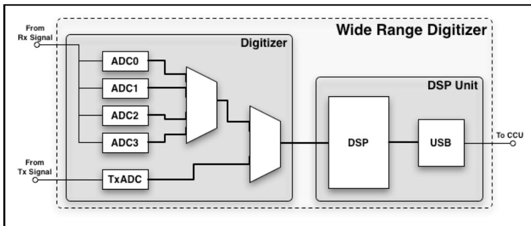
Figure 1. A block diagram representing the WRD system.
