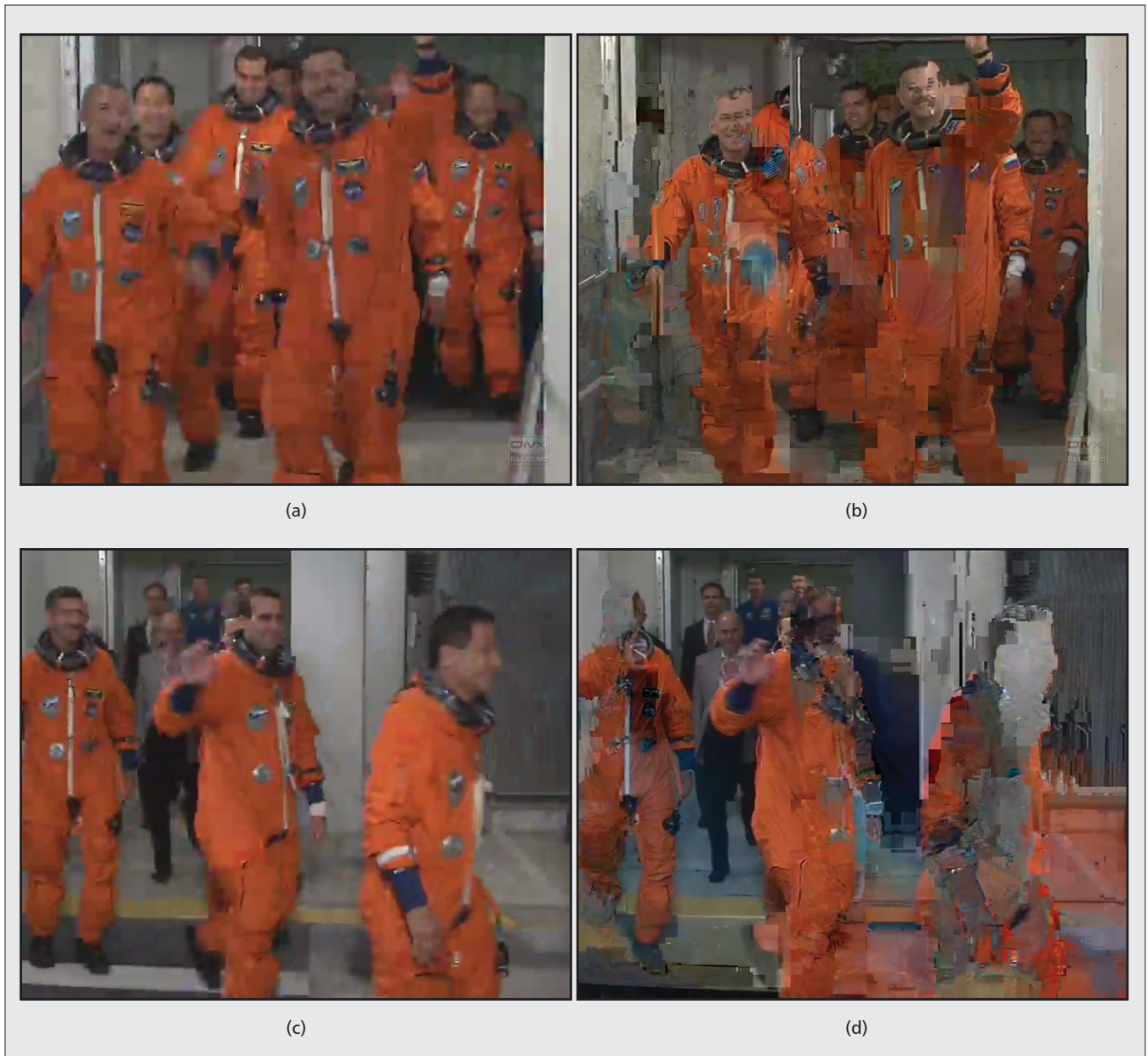
Figure 3. 100th and 250th frames with and without rate control: a) 100th frame with rate control; b) 100th frame without rate control; (c) 250th frame with rate control; d) 250th frame without rate control.
