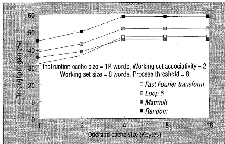
Figure 11. Uniprocessor throughput gains versus operand cache size.
