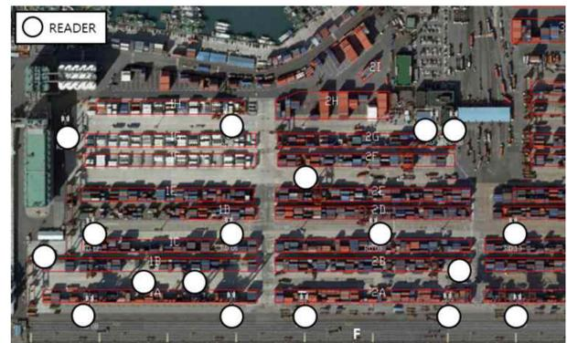
Fig. 16 Target Environment and reader installation
