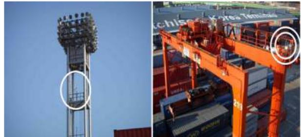
(b) RFID Readers on the top of light tower and transfer crane
