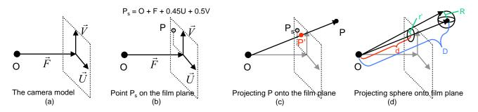
**Figure 3:** (a) The Four-point camera model is constructed from an eye point, a vector to the film plane, and two vectors which span the film plane. (b) An image-space constraint p is converted to a 3D point  $P_s$  on the film plane. (c) Projecting P onto the film plane (P'). (d) For the scale constraint, the radius r of the projected circle is found by scaling the radius R of the bounding sphere by the ratio of the distance from the eye to P'.
