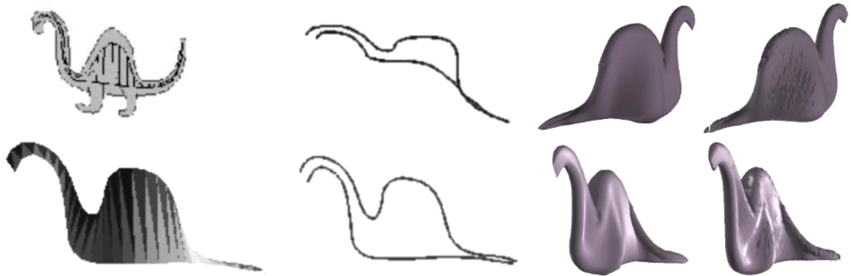
Figure 11: A surface which is difficult to do with a single axis curve, but simple to do with a ruled surface axis. Left: A sketch of this type of surface and the ruled axis constructing it with the actual ruled surface below. Middle left: The two axis curve viewed from above and the side. Middle right: The parametric approximation. Right: The implicit surface. This surface was made with 6 profile curves
