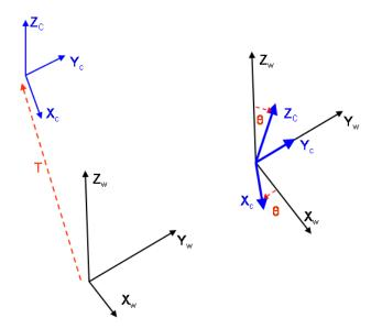
Figure 3.3: Extrinsic Properties of the Camera.
