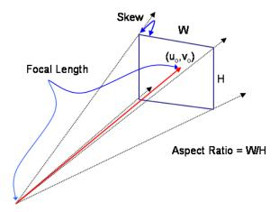
Figure 3.4: Intrinsic Properties of the Camera.
