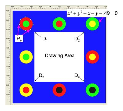
Figure 3.1: Calibration pattern with chromaglyphs. The points  $D_{1-4}$  are the corners of the drawing space. The points,  $P_e$ , are the known points on the ellipse borders. The circles in the pattern can be represented by equations of the form above.
