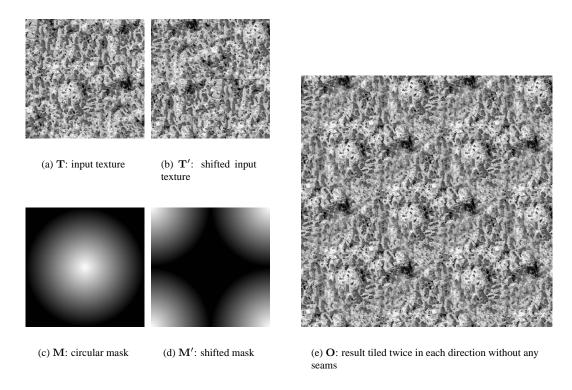
Figure 3. Generating a tileable texture level.
