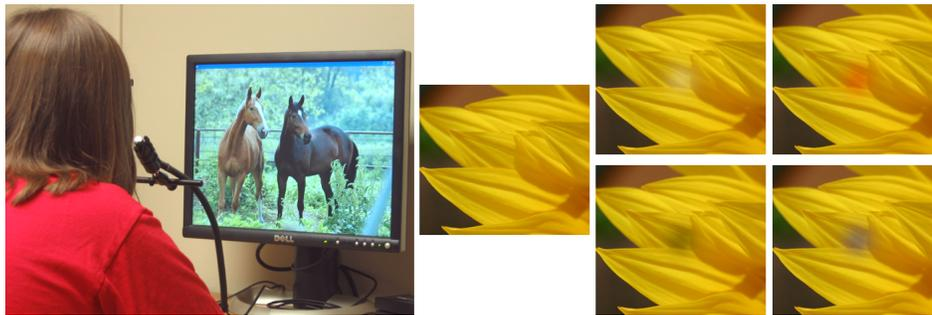
Fig. 3. Photograph of experiment setup (left). Small patch from a test image (center). Example of luminance modulation (third column). Example of warm-cool modulation (right column).
