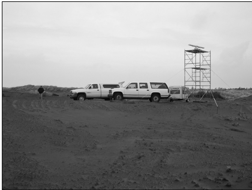
Figure 31 - X-band remote sensing system set up for the MCR field deployment.
