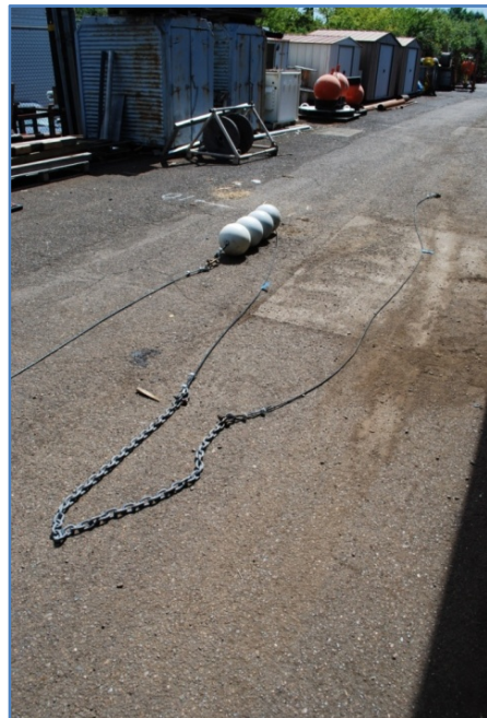
Figure 27: Upper portion of Strawberry Hill mooring
