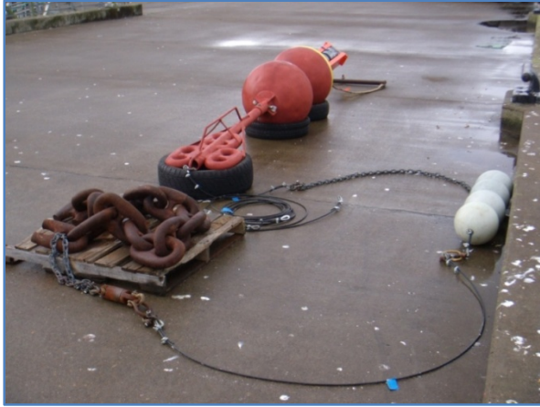
Figure 28: Fully Assembled mooring laid out on the pier
