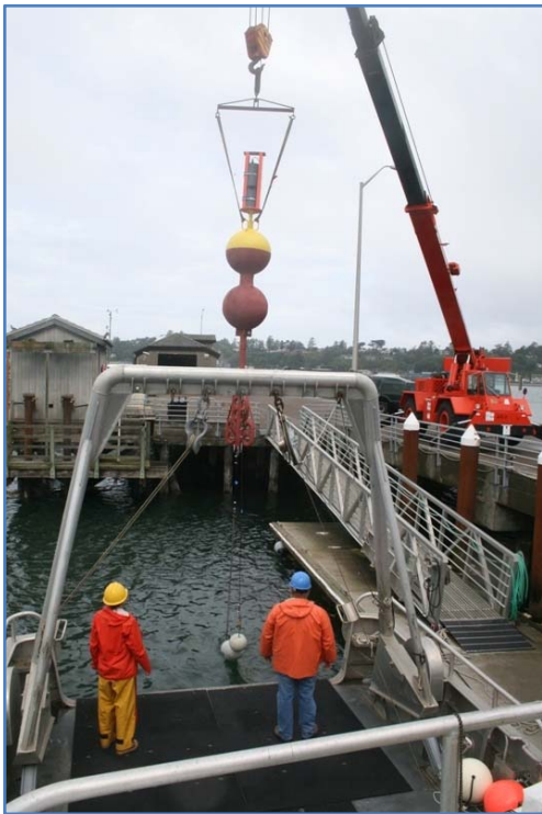
Figure 30: Lowering the buoy into Yaquina Bay
