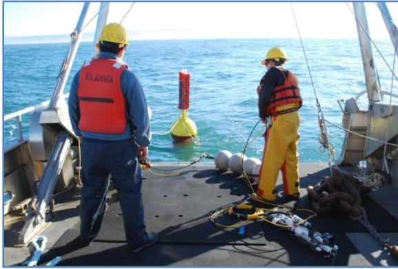
Figure 40: Paying out the mooring while trolling the buoy
