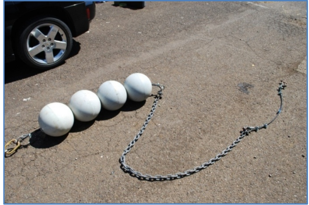
Figure 25: Upper portion of Yaquina Bay mooring
