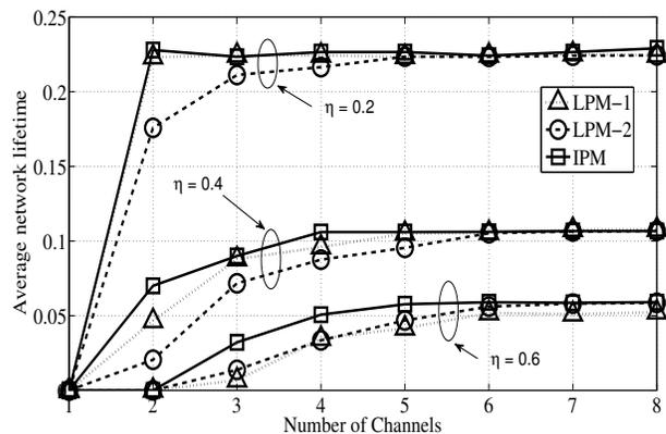
Fig. 5. Average network lifetime (hour) for  $r = 30m$ ,  $|\mathcal{N}| = 30$ , and  $\mathcal{A} = 100 \times 100 m^2$ .
