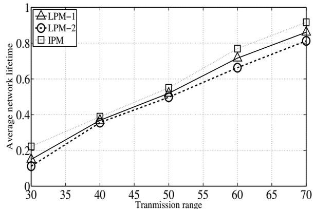
Fig. 4. Average network lifetime (hour) for  $|\mathcal{N}| = 30$ ,  $\mathcal{A} = 100 \times 100m^2$ , and  $c = 3$ .
