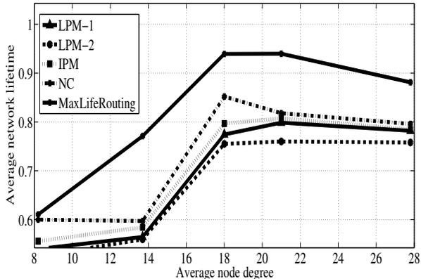
Fig. 7. Average network lifetime (hour) for  $r = 30$ ,  $\mathcal{A} = 100 \times 100m^2$ , and  $c = 1$ .
