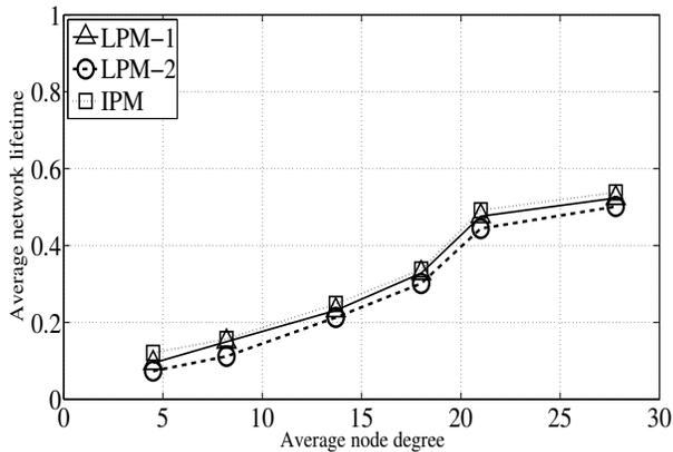
Fig. 3. Average network lifetime (hour) for  $r = 30m$ ,  $\mathcal{A} = 100 \times 100m^2$ ,  $\eta = 0.3$ , and  $c = 3$ .
