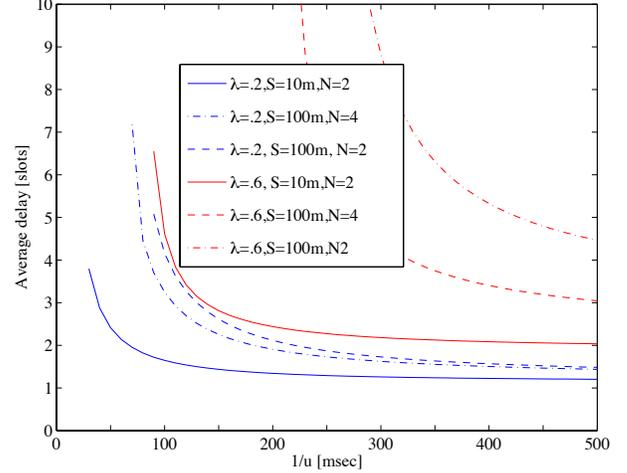
Fig. 10. Average delay vs average of channel availability time ( $\bar{T}_{idle}$ )
