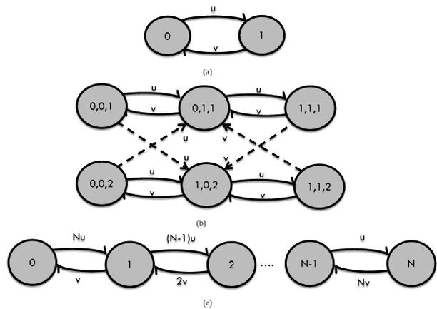
Fig. 2. (a) Single channel Markov chain. (b) Extended model of the two-channel availability. (c) Simultaneously occupied channels model.
