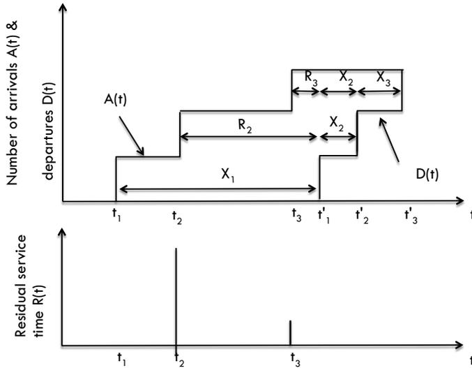
Fig. 3. The concept of residual service time
