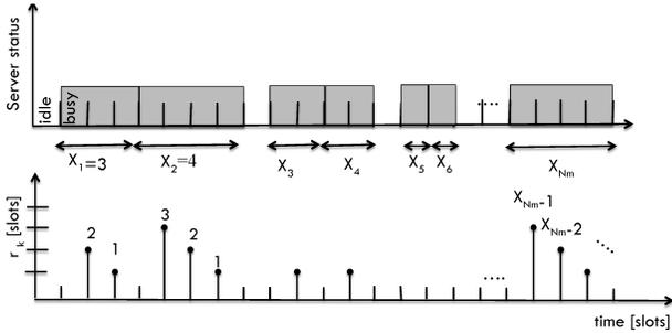
Fig. 4. A sample path of a server status and the corresponding residual service time.
