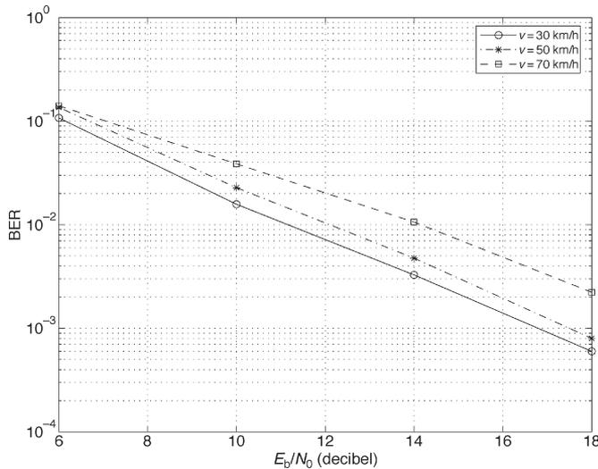
Fig. 4. BER versus  $E_b/N_0$  with different fading rates.
