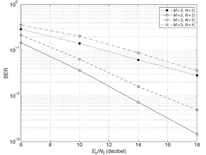
Fig. 3. BER versus  $E_b/N_0$  for a different number of transmit and receive antennas.
