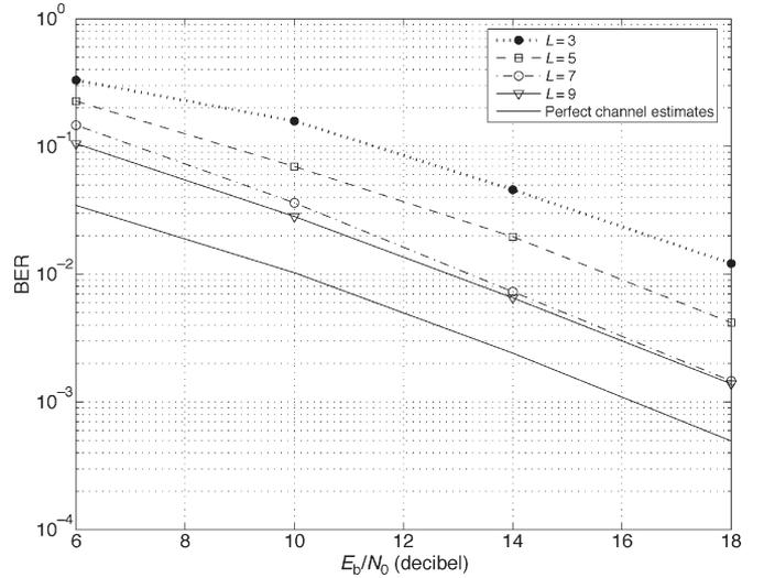
Fig. 2. BER versus  $E_b/N_0$  with different memory depth  $L$ .
