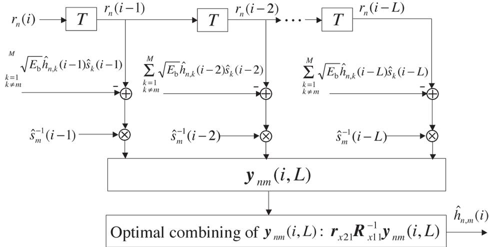
Fig. 1. The DD MAP channel predictor for MIMO systems.
