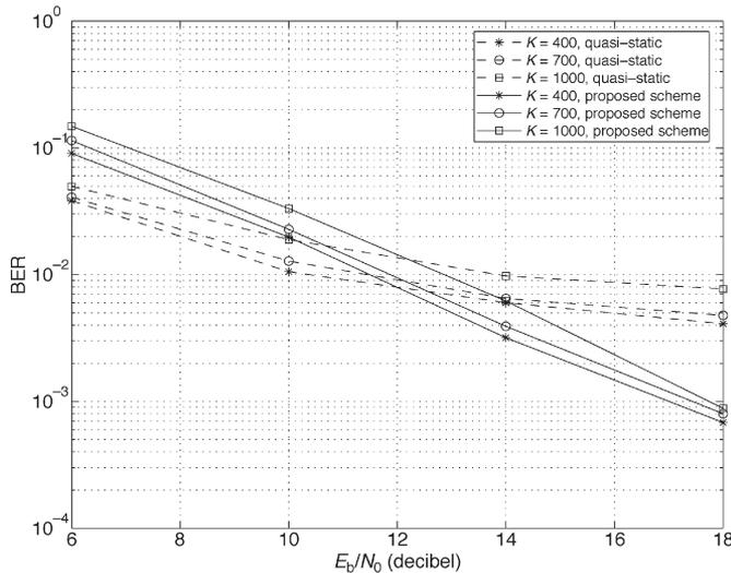
Fig. 5. Performance comparison of the proposed scheme and the scheme with the channel treated as block fading.
