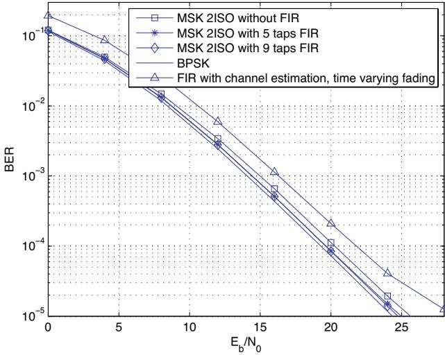
Fig. 4. Performance of space-time block coded GMSK ( $BT = \infty$ ,  $L = 1$ ,  $M = 2$ ).
