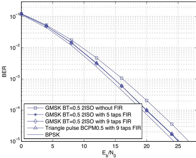
Fig. 5. Performance of space-time block coded GMSK ( $BT = 0.5$ ,  $L = 2$ ,  $M = 2$ ).
