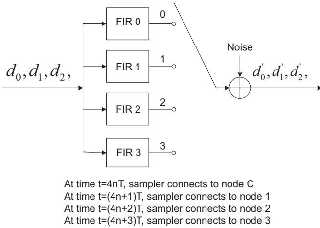
Fig. 3. Equivalent system model for space-time block coded GSMK with 4 antennas.
