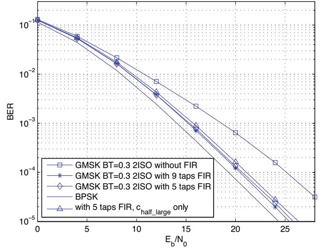
Fig. 6. Performance of space-time block coded GMSK ( $BT = 0.3$ ,  $L = 3$ ,  $M = 2$ ).
