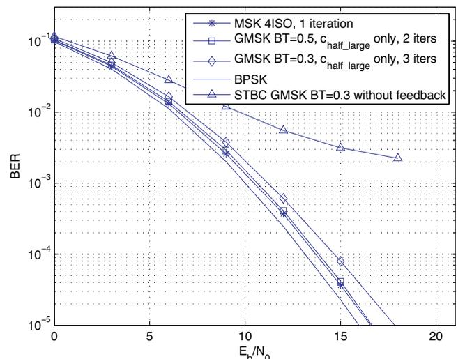
Fig. 7. Performance of space-time block coded GMSK with 4 transmit antennas.
