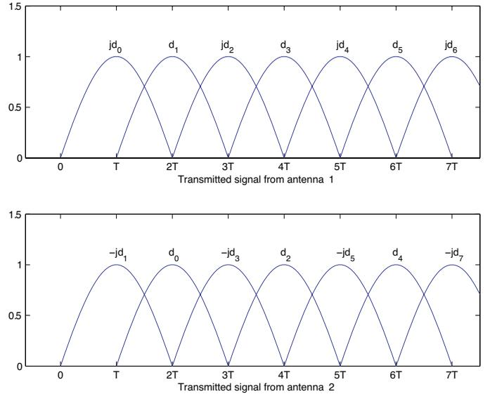
Fig. 1. The modified Alamouti scheme ( $M = 2$ ) for MSK with precoding based on Laurent decomposition.
