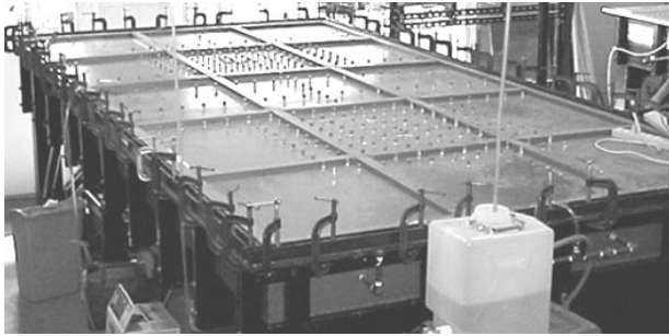
Figure 1. Photograph of physical aquifer model (PAM) used in laboratory tests.
