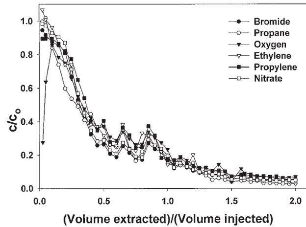
**Figure 2.** Extraction phase breakthrough curves for short-term transport test showing conservative transport of dissolved gases and nitrate.
