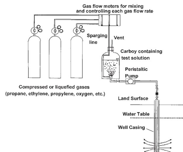
Figure 1. Field setup for single-well push-pull tests.
