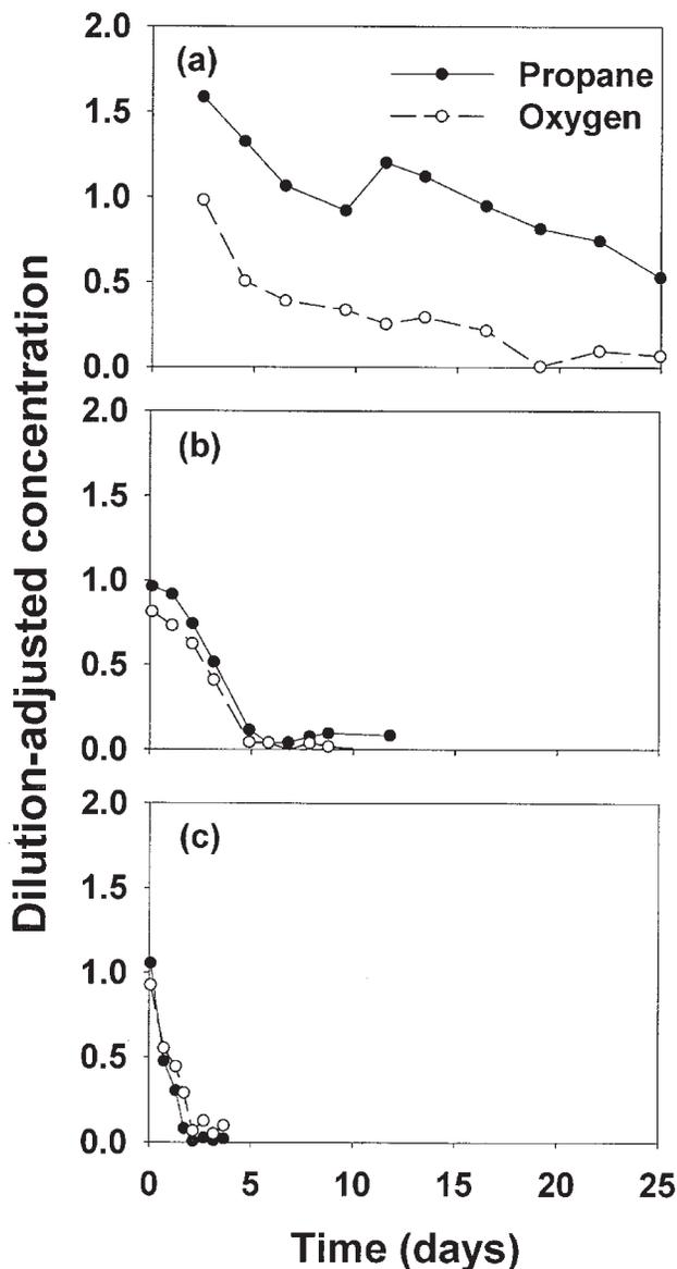
**Figure 3.** Dilution-adjusted propane and oxygen concentrations during the (a) first, (b) second, and (c) third biostimulation tests.
