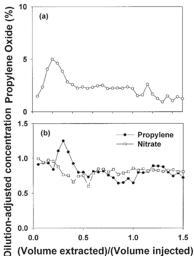
**Figure 6.** (a) Propylene oxide concentrations in the extracted ground water as a percent of average propylene concentration in injected test solution; (b) dilution-adjusted concentrations for propylene and nitrate during propylene activity test.
