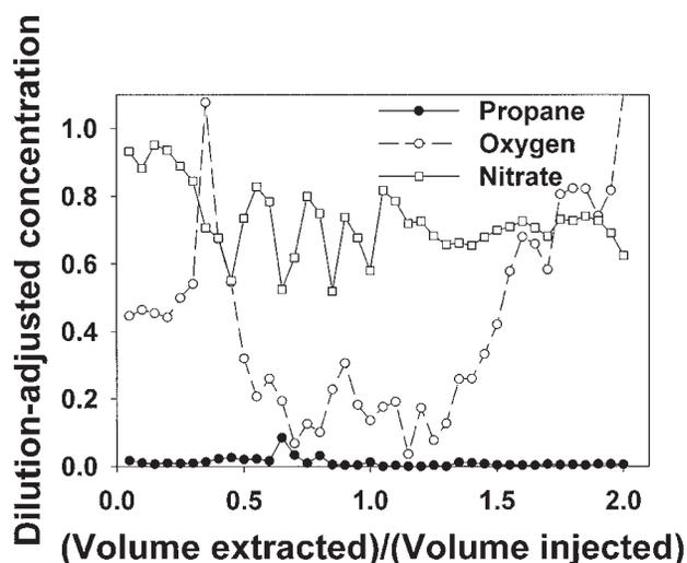
**Figure 4.** Dilution-adjusted concentrations of injected propane, oxygen, and nitrate during propane activity test.
