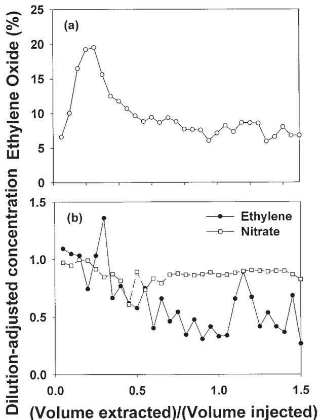
Figure 5. (a) Ethylene oxide concentrations in the extracted ground water as a percent of average ethylene concentration in injected test solution; (b) dilution-adjusted concentrations for ethylene and nitrate during ethylene activity test.
