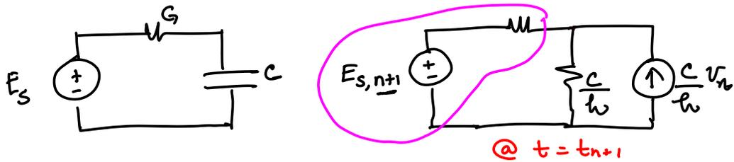
Given an initial condition across the capacitor  $v_0$
