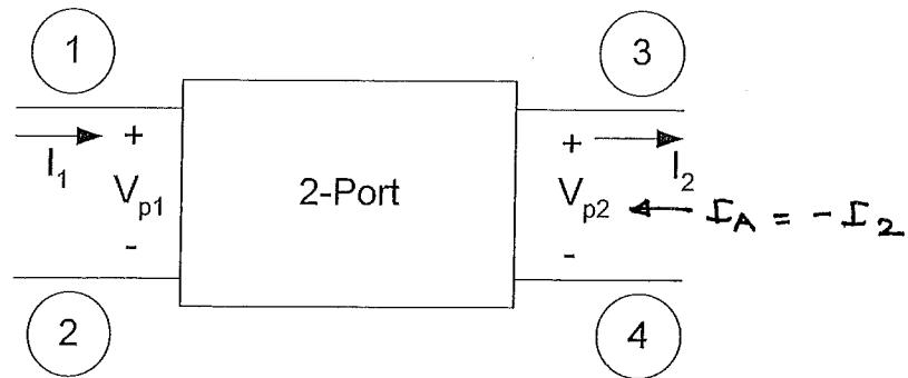
The  $ABCD$ -parameters are defined as (note the direction of  $I_2$ )
