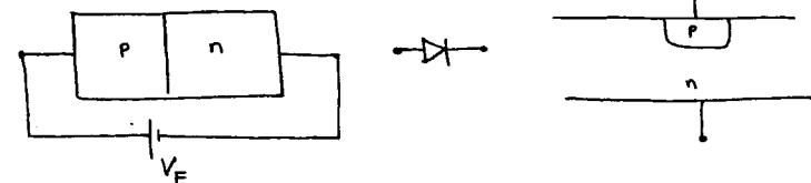
For a forward voltage  $V_F > 0$  current I is given by
