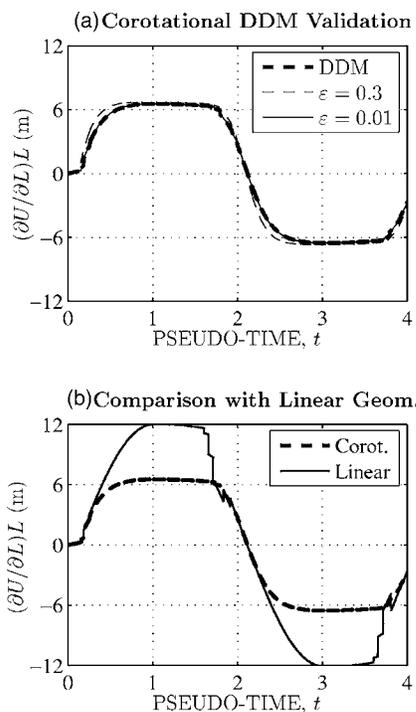
**Fig. 10.** Response gradient of slender steel cantilever computed with respect to the cantilever length: (a) validation of the corotational DDM computation by finite differences; (b) comparison of corotational gradient with that for linear geometry
