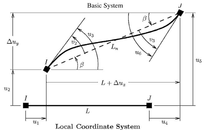
Fig. 2. Geometric transformation between the local coordinate system and the basic system
