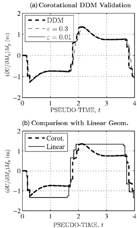
**Fig. 11.** Response gradient of slender steel cantilever computed with respect to the yield moment: (a) validation of the corotational DDM computation by finite differences; (b) comparison of corotational gradient with that for linear geometry
