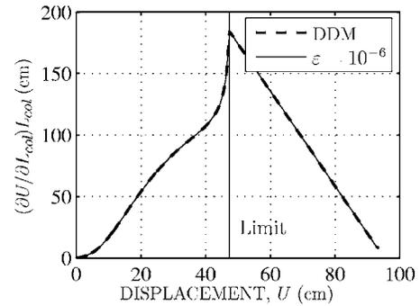
**Fig. 7.** Response gradient of Lee's frame computed with respect to the column length by the direct differentiation and finite-difference methods
