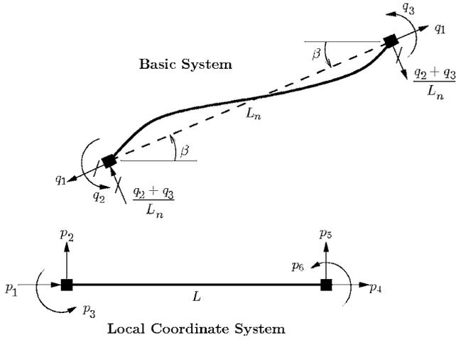
**Fig. 3.** Equilibrium transformation between the basic system and the local coordinate system
