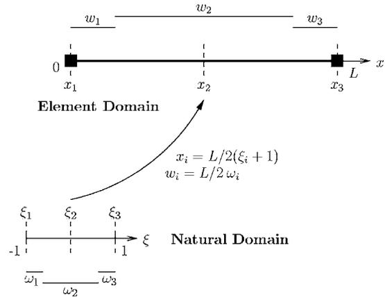
Fig. 4. The mapping of integration points from the natural domain to the element domain for three-point Gauss-Lobatto quadrature
