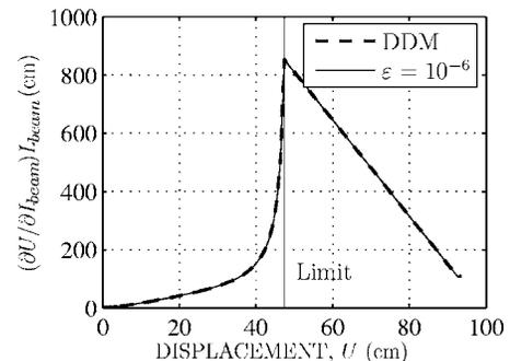
**Fig. 8.** Response gradient of Lee's frame computed with respect to the beam length by the direct differentiation and finite-difference methods
