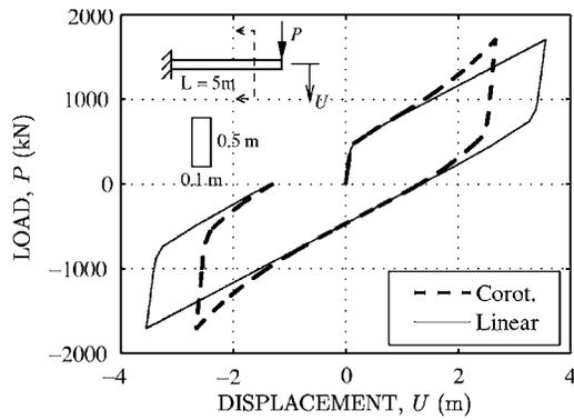
**Fig. 9.** Load-displacement response of slender steel cantilever using one force-based element considering small displacement linear geometry and large displacement nonlinear geometry according to the corotational theory
