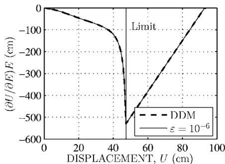
**Fig. 6.** Response gradient of Lee's frame computed with respect to the material modulus of elasticity by the direct differentiation and finite-difference methods
