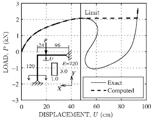
**Fig. 5.** Load-displacement response of Lee's frame computed with a load-control incremental solution strategy
