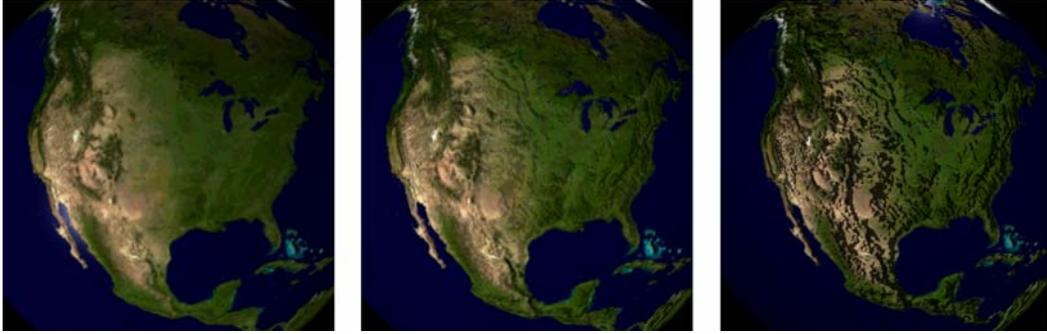
**Figure 13: Successively increasing bump-map scaling. The left image (no bumpmapping) looks flat, while the middle image looks good. From this camera viewpoint, bumpmapping is indistinguishable from displacement mapping.**
