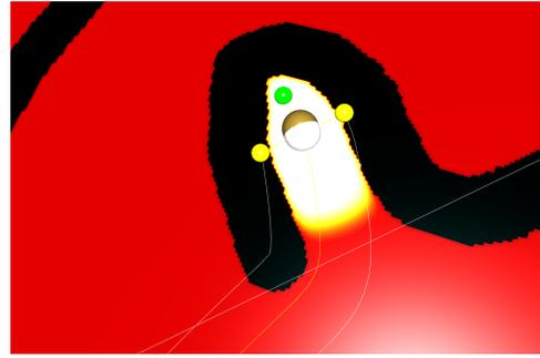
Fig. 10. A goal directed activity field rendered in heated object color scale, with a tractor travelling towards the goal.
