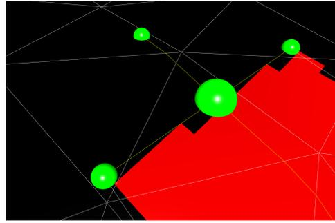
Fig. 5. Our simplified model of a tractor, the large sphere represents the the center of the tractor, while the smaller two the left and right represent the endpoints of the “plow,” the forward sphere indicates direction, and can be used for sampling of data ahead of the tractor. The red areas indicate “covered” terrain.
