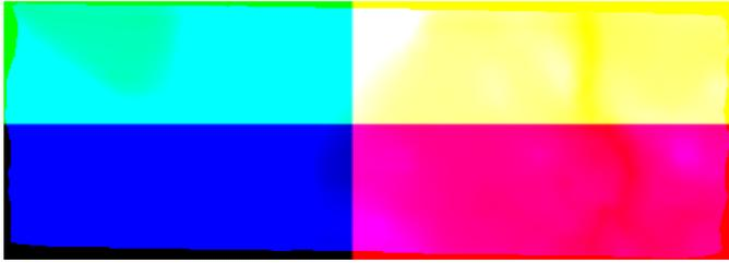
Fig. 3. A discretized farm field rendered to a texture, the  $\langle x, y, z \rangle$  coordinates of the terrain are mapped to the  $\langle r, g, b \rangle$  color channels of a floating point texture.
