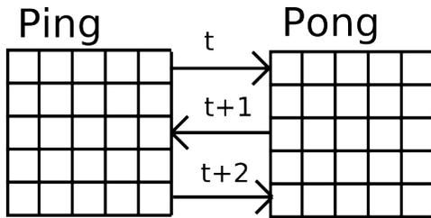
Fig. 4. Ping & Pong represent two textures bound to the framebuffer, they are alternately the input to and output of the shunting equation, allowing the neural activity to be iteratively propagated through time.
