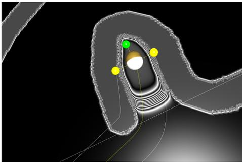
Fig. 8. Contour lines on a goal-directed activity field with obstacles.
