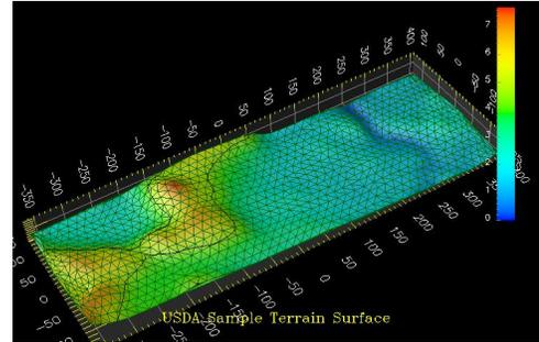
Fig. 2. The terrain data arrives as an untriangulated collection of scattered Digital Elevation Map (DEM) points.
