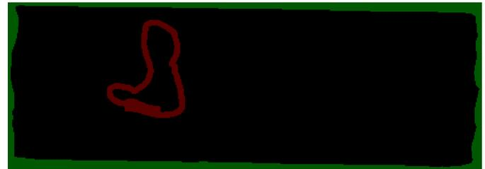
Fig. 6. Sample contour-directed coverage texture, covered areas are in red, obstacles are in green, and black represents uncovered terrain.
