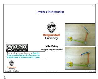
**Inverse Kinematics** Forward Kinematics solves the problem "if I know the link transformation parameters, where are the links?". **Inverse Kinematics** (*IK*) solves the problem "If I know where I want the links to be (X\*,Y\*), what link transformation parameters will put them there?" (X\*,Y\*) Ground
