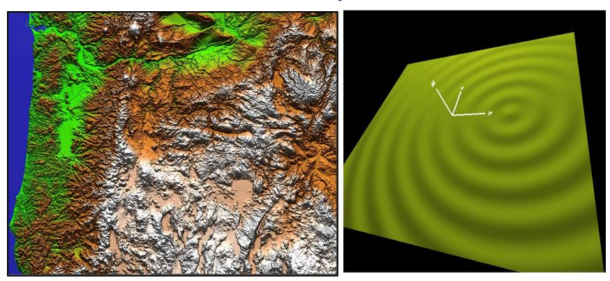
Height Field bump-mapping is straightforward because the underlying coordinate system is constant. Each fragment's Z points up, each fragment's X points right, etc. Thus, the tangent vectors always involve  $\frac{dz}{dx}$  and  $\frac{dz}{dy}$ .
