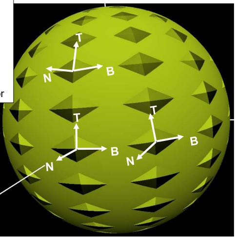
We will assume that we know the Normal everywhere because of how the shape was modeled. Now, how do we find T and B? And, how do we convert these to X-Y-Z?
