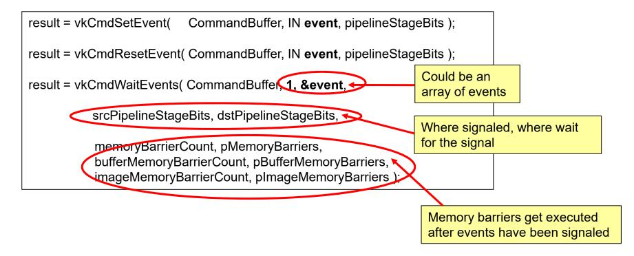
Note: the GPU cannot test for an event, but it can block waiting for one
