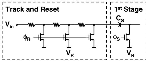
Fig. 5. Input track and reset
