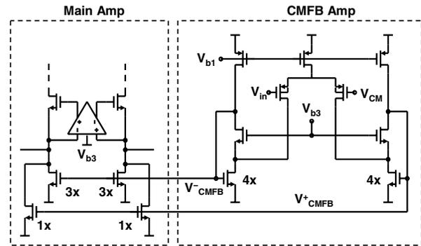
Fig. 7. CMFB loop gain reduction using positive feedback
