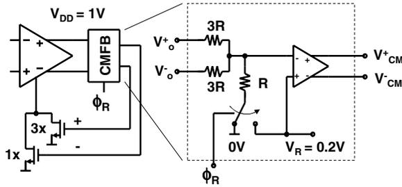
Fig. 3. Switching common-mode feedback
