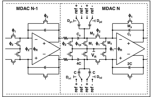
Fig. 4. Fully differential ORST MDAC for a pipelined ADC
