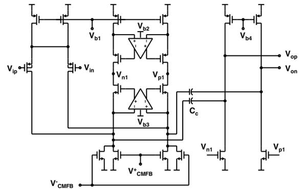
Fig. 6. Two-stage, gain boosted opamp
