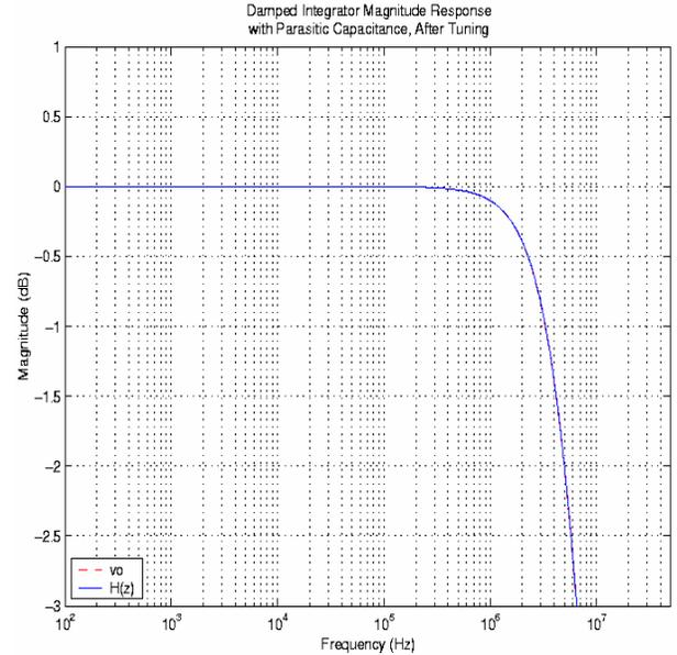
Fig. 5: Magnitude response of damped unity-gain buffer SC integrator with parasitic capacitance after tuning.
