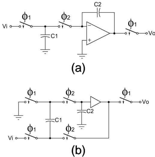
Fig.2: SC Integrators: (a) Conventional; (b) Unity-gain buffer.
