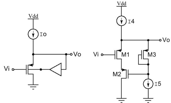
Fig. 1: PMOS Source Followers: (a) PMOS SF with n-well buffer; (b) cascoded PMOS SF.
