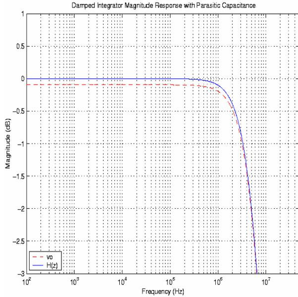
Fig. 4: Magnitude response of damped unity-gain buffer SC integrator with parasitic capacitance.
