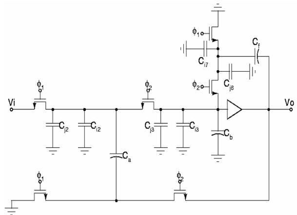
Fig.3: Damped unity-gain buffer SC integrator with stray capacitance.
