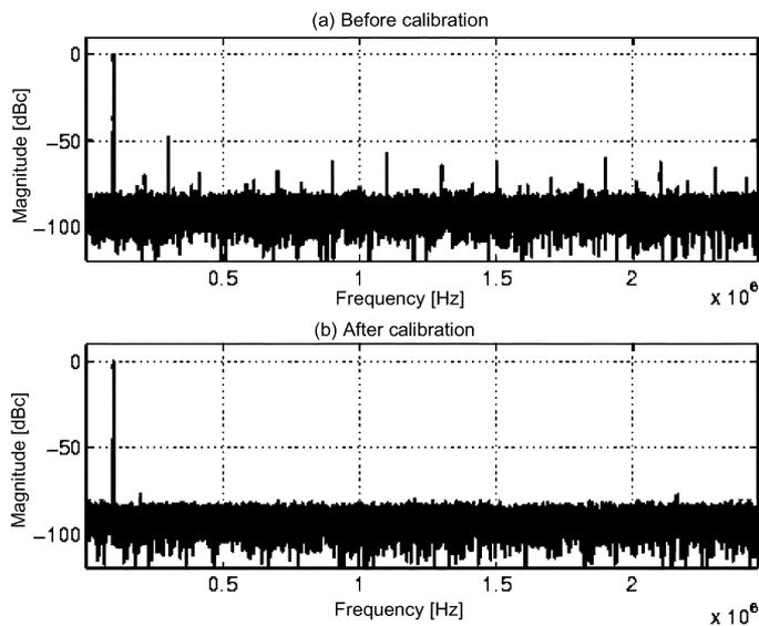
Fig. 17. Measured ADC output spectrum at 5 MSPS.
