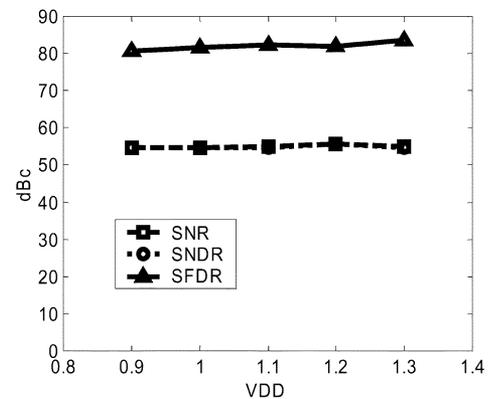
Fig. 19. Dynamic performance versus power supply voltage.
