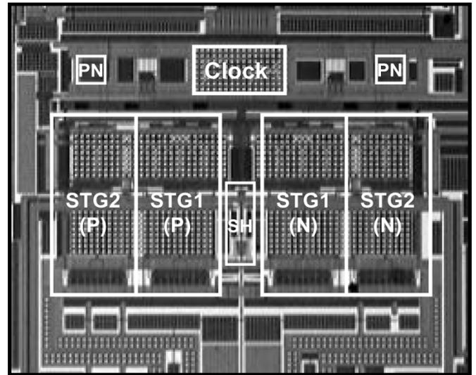
Fig. 14. Die photograph of the prototype ADC.
