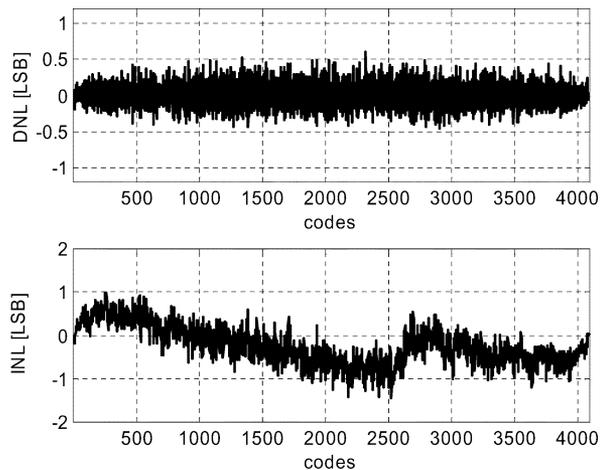
Fig. 16. DNL and INL after calibration.
