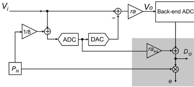
Fig. 3. Background equivalent radix extraction.
