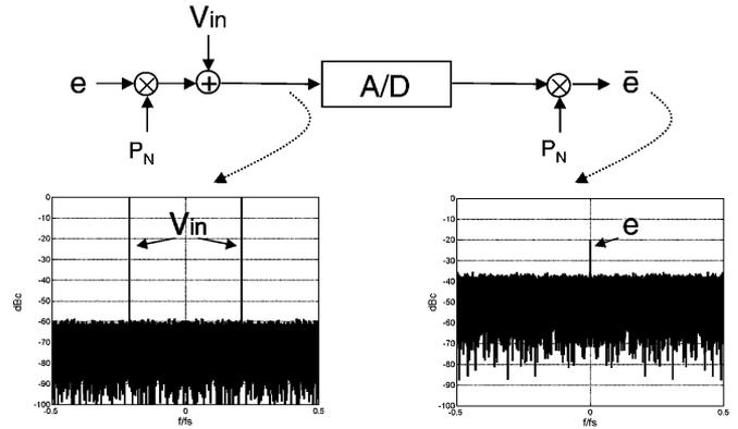
Fig. 4. Interference from the input signal.
