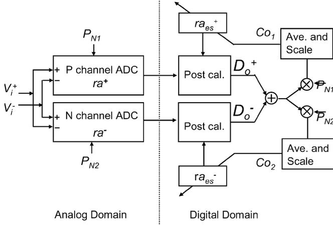
Fig. 5. Overall ADC with proposed background digital calibration.
