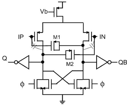
Fig. 12. Static latched comparator.
