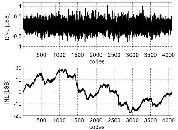
Fig. 15. DNL and INL before calibration.
