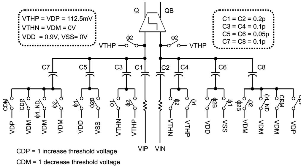
Fig. 11. Low-voltage SC comparator with dithering.
