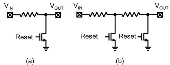
Fig. 10. Passive track-and-reset circuit MDAC.
