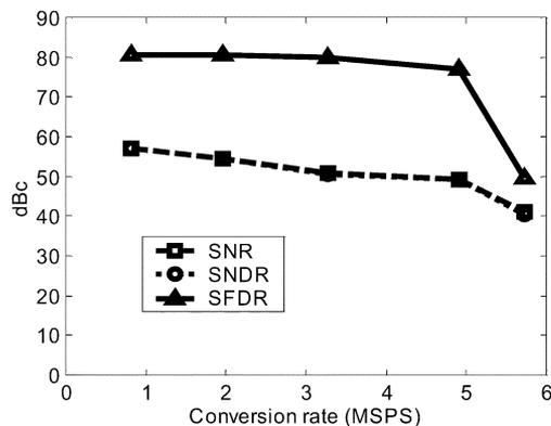
Fig. 18. Dynamic performance versus conversion rate.
