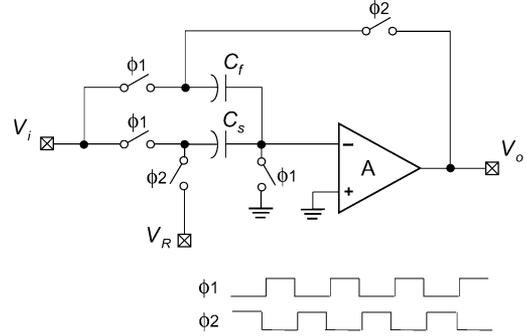
Fig. 2. Capacitor-flip-over MDAC.
