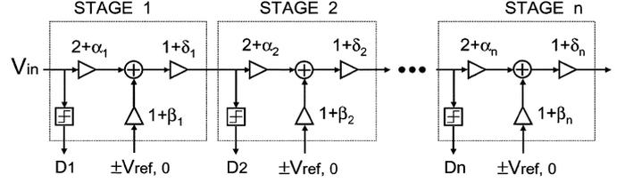
Fig. 1. Functional diagram of a pipeline ADC (1.5 bit per stage).
