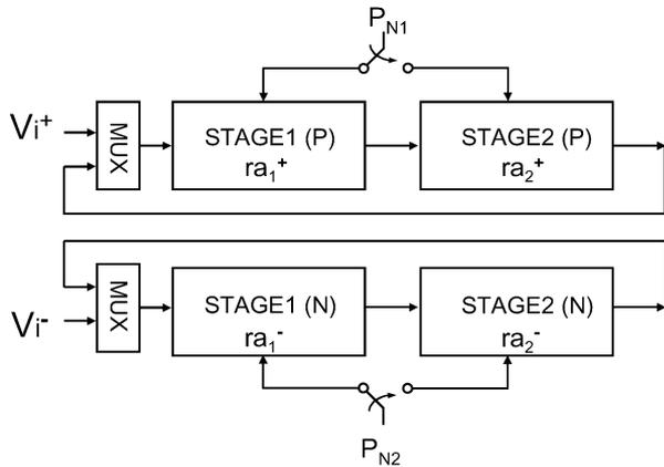
Fig. 6. Two-stage algorithm ADC with calibration.
