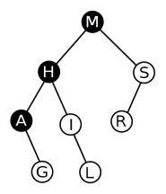
Let's traverse the treap by using inorder sequence. Then, the sequence is sorted by keys increasingly. Set the sequence as nodes[1..n]. Then, we know that nodes[i].key<nodes[j].key if and only if i<j. In Jeff Ericksons lecture 10, we know that if nodes[i] is parent or ancestor of nodes[j](i!=j), nodes[i] should have the smallest priority among nodes[i..j](if i < j) or nodes[j..i](if i > j). This lemma is not proved in this problem.
