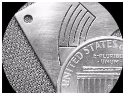
Figure 3: Serpentine spring cut with CO 2 laser machining of stainless steel (after clean up). Shim thickness is 250 \mu\text{m} .
