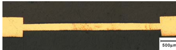
Figure 7: \Delta CTE Bonded Sample Showing Minimal Fin Warpage
