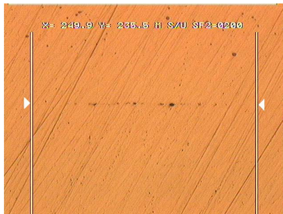
Figure 9: Bond Line Hot Press (800°C/6MPa/30min)
