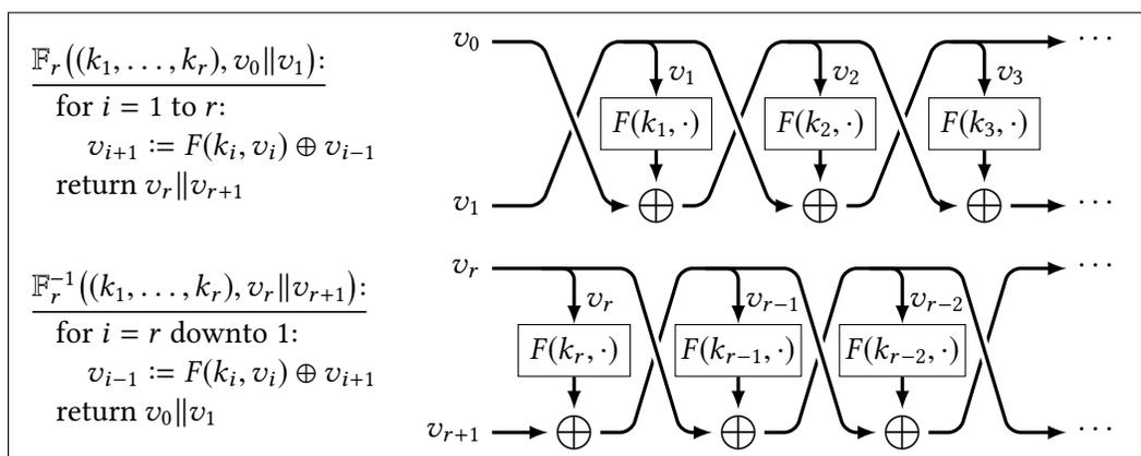
Because each round is invertible (given the appropriate round key), the overall Feistel cipher is also invertible. Note that the inverse of the Feistel cipher uses inverse Feistel rounds and reverses the order of the key schedule.
